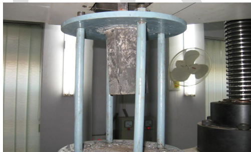
Fig.10. Formation of longitudinal splitting cracks
